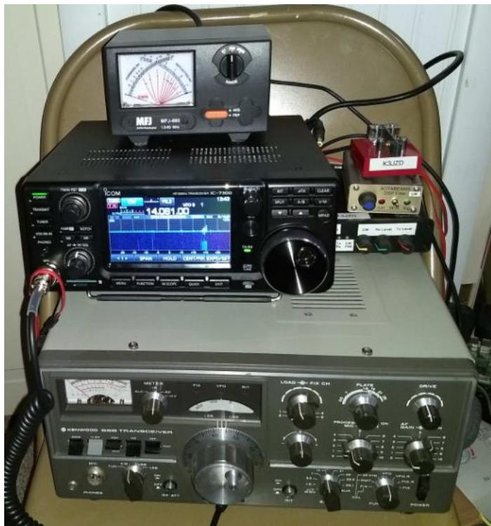
lights. But in all fairness, the TS-520S has an internal power supply and is all ready to plug into 120VAC whereas the 7300 needs an external power supply.
