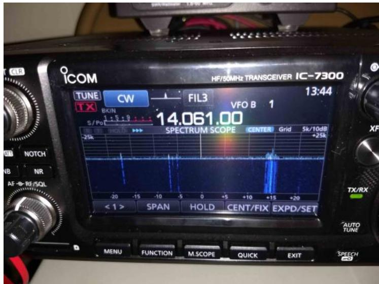
screen layout so that the bandscope and waterfall take up more than 50% of the screen height, and that it was also very easy to adjust the displayed frequency range. If I had to criticize, I would say that the 'soft buttons' that are on the bottom of the screen that allow you to make these adjustments are a bit too large. I would rather see smaller buttons and a little more waterfall history.
